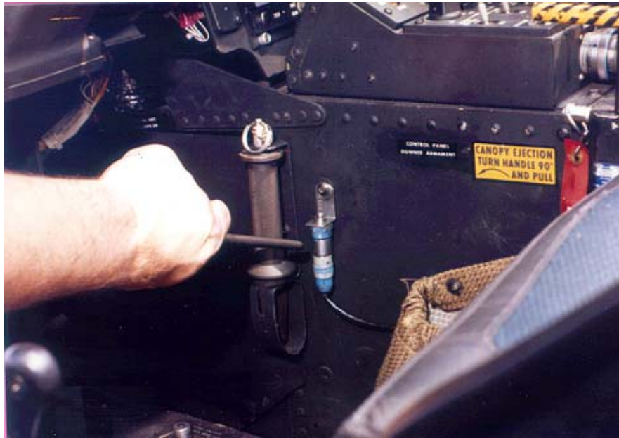
Figure 5. Vertical Accelerometer Installation Near Canopy Removal Arm and Fire Mechanism
