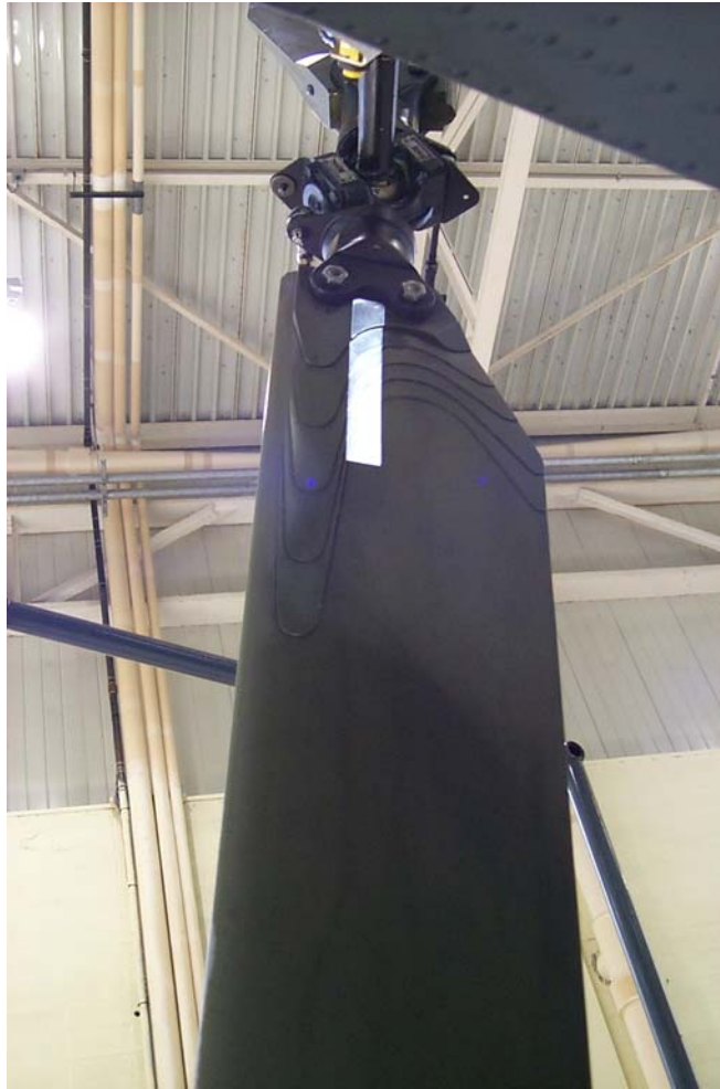
Figure 9. Tail Rotor Reflective Tape
