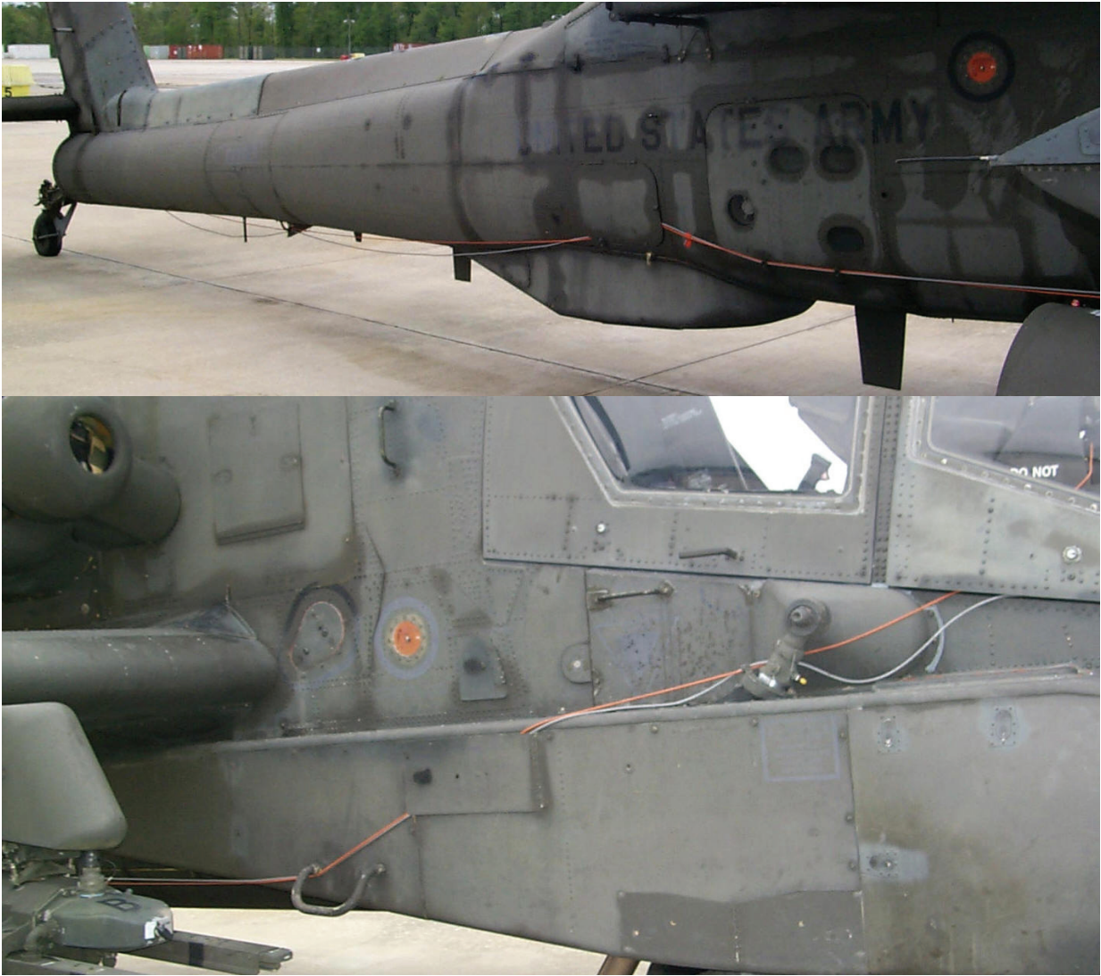
Figure 15. Tail Accelerometer Cable Routing
