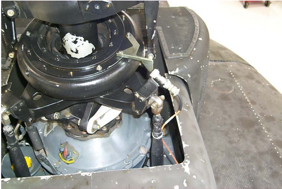
Figure 3. Magnetic RPM Sensor Installation
