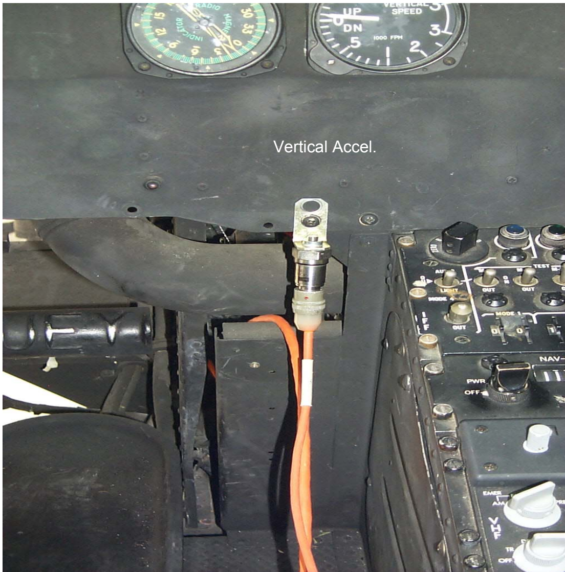
Figure 5. Vertical Accelerometer Installation on Instrument Panel
