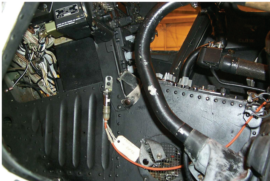
Figure 4. Vertical Accelerometer Installation
