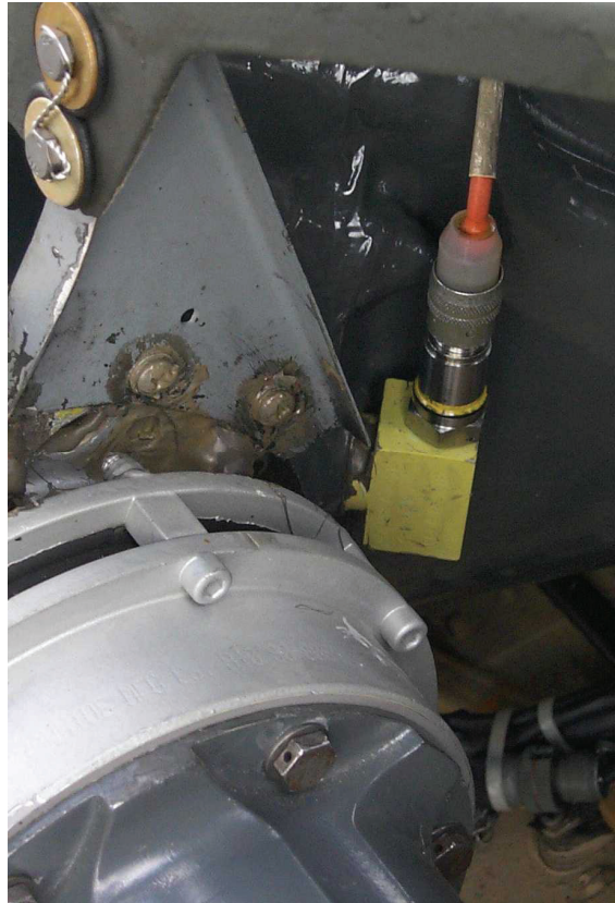
Figure 18. No. 1 Input Module Accelerometer Installation (ACC1)
